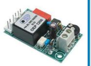
Amplifier on board for increasing the output volume of the internal loudspeaker or to connect an external loudspeaker
