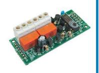
Board with 2 relays (to switch door lock, lights, etc.) for remote or local control through programmable codes
