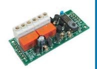
Board with 2 relays (to switch door lock, lights, etc.) for remote or local control through programmable codes
