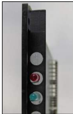
Figure: TMDID – LEDs on the Front Panel
