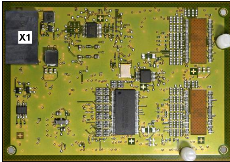
Figure: OCCB3 - component side with inserted spacing bolts
