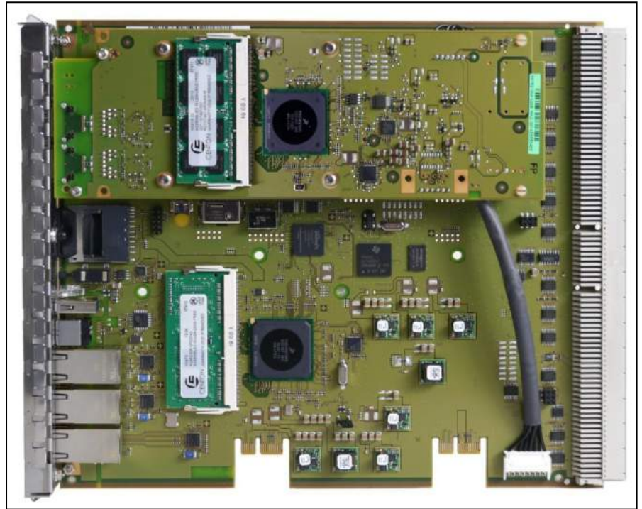
Figure: UC Booster Card OCAB mounted on OCCL
