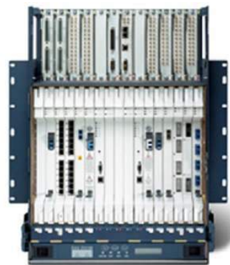
Figure 2. Cisco ONS 15454 ETSI/SDH System
