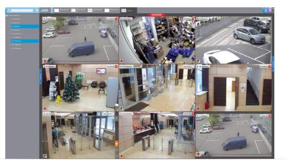
The new Alarms Panel is implemented as a drop-down resizable window (and can be expanded to full screen). The alarms panel displays video thumbnails of recent alarms that require operator attention. Advantages of the new panel include customization of the size of the panel and alarm thumbnails, based on the number of events to be displayed. In addition to current (unclassified) alarm events, the panel allows viewing previously processed alarms.
