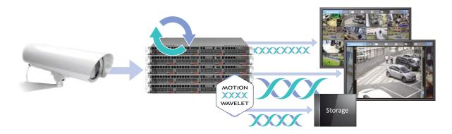
**MotionWavelet** is an efficient video codec based on wavelet conversion, providing more flexible selection of the quality of video to stream to remote clients. It is best used with with Green Stream.
