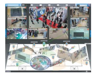
The interactive 3D map is a set of ordinary raster blueprints for a site, placed on the screen under viewing tiles, which are displayed in a lifelike projection. On the map you can indicate the location of the cameras included in the layout, as well as mark sensors and detectors. Click a viewing tile to immediately see where the relevant camera is located on the map.
